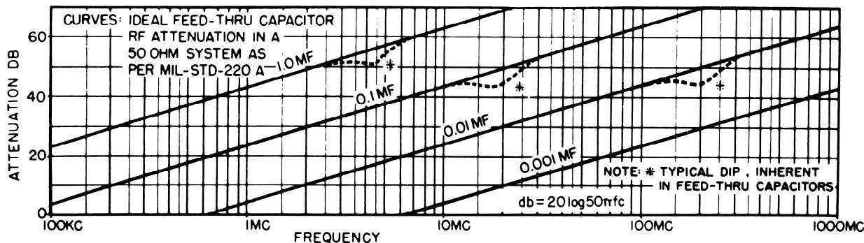
These units designed to meet all electrical, mechanical and environmental requirements of MIL-C-11693 for feed-thru suppression capacitors.
